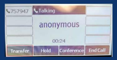
Whilst on an active call, press the transfer key - This places the call on hold
